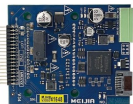
美嘉星光新系统头板 FRONT BOARD FOR MEIJI INKJET NEW DIMATIX SYSTEM
